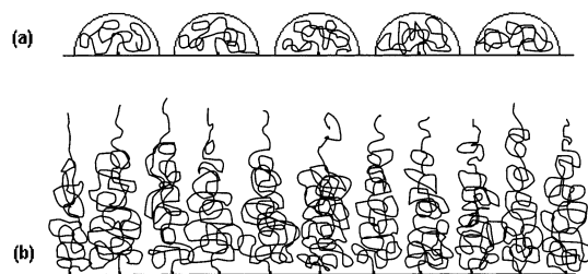
Figure 1. Drawings of tethered layer conformations as predicted by theory. (a) The mushroom layer consists of nonoverlapping, coiled tethered chains, and (b) the brush layer consists of crowded, stretched tethered chains.
